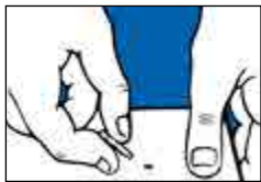
1. Insert receptacle into the drill hole.
