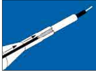
2. Insert prestripped wire into notch on FIT tool and slide until it protrudes approximately 1/8 inch from insulator.
