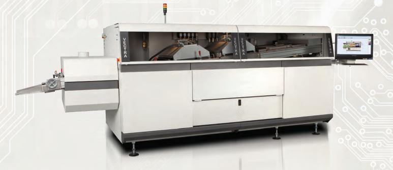
The Electrovert VectraElite is an ideal wave soldering solution for medium-to-high mass board assemblies in a soldering environment that requires fast changeover, process flexibility, and system reliability.
